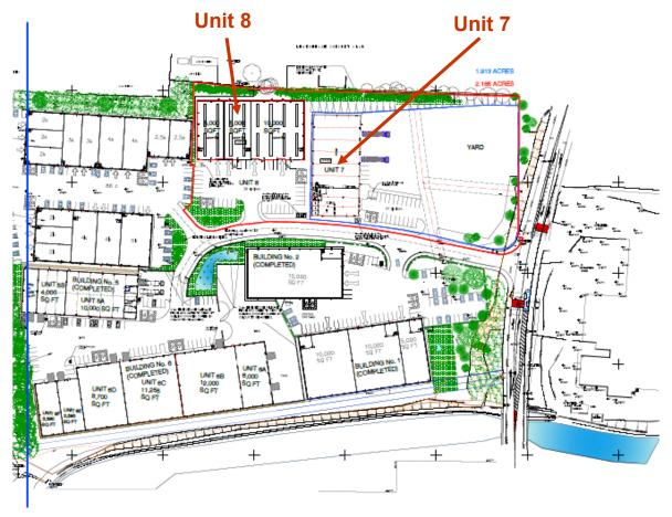
The proposed units would be constructed with buff brickwork to the lower walls and profiled steel cladding to the roof and walls in goosewing grey with darker grey trimming. Unit 7 would have a ridge height of 8.2m and Unit 7 which is sited in the north west corner of the site would have a ridge height of 8.0m. A partial mezzanine would be installed at Unit 7 to be used for additional storage.
